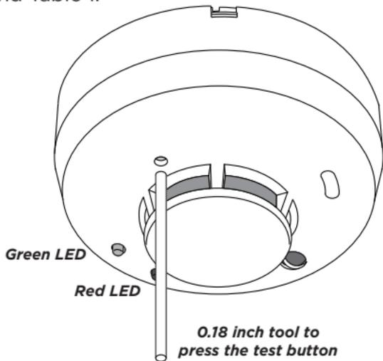
**Figure 6: Test Button Location**
