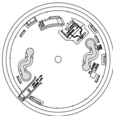
**Figure 3: Mounting Hole Locations**
