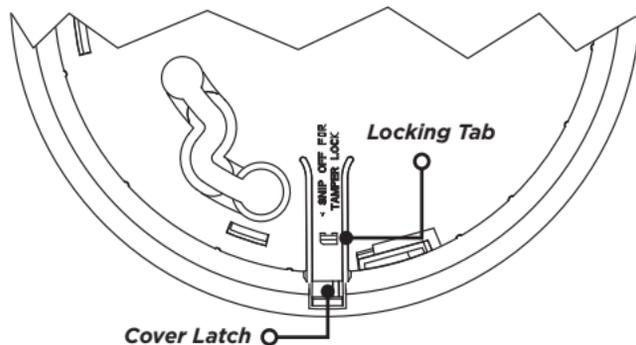
**Figure 4: Mounting Base and Tamper Switch**
